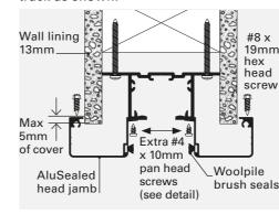
Spot through the pre drilled hole in the flange with a Ø2.5mm drill into the bottom of the track.
