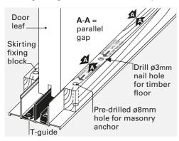
(See red stamped arrow on the timber). To **timber** floors: Use Ø3.15mm x 75mm nails on either side in the centre of the skirting fixing block thickness. (See the red stamped ⊕ on the timber). Pre-drill Ø3mm holes for these nails.
