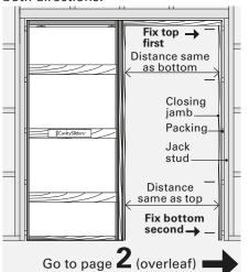
AluSealed units: Screw through pre-drilled holes in the centre of the closing jamb.
