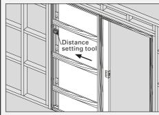
The rear activator is now positioned. Securely tighten all four grub screws.
