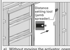
e) Without moving the activator, open the door and securely tighten all four grub screws.
