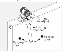
Note: The top of the hanger pin screws into a self-locking Nyloc type nut in the carriage. For the assembly to remain in its adjusted position over time the hanger pin must be screwed into the nylon locking portion of the nut by at least 3 full turns.
